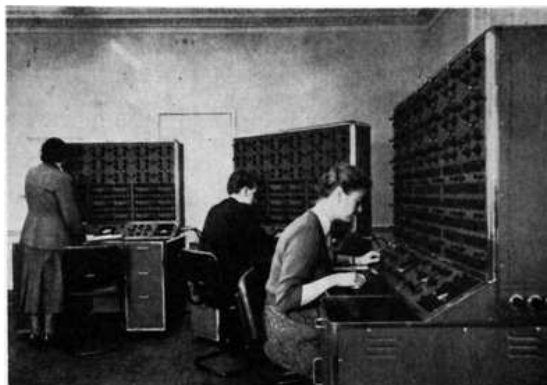
Fig. 3—Three Short computers in service with Vickers Armstrongs (Supermarine) Ltd. They are used for investigation of aircraft flutter and stability problems—Short Brothers
